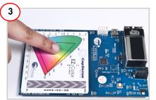
Tap the color gamut to view different colors from the RGB LED. Adjust the brightness using the slider available to the right of the gamut.
