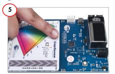
To put the board to "sleep" while powered, press and hold the circular emblem to the left of the CapSense logo.
