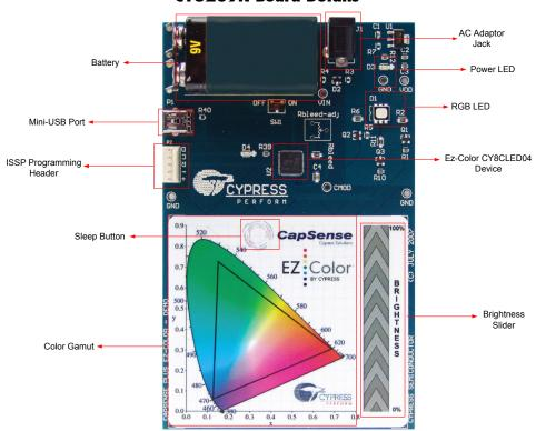
Note: For optimum performance, place the board horizontally on a flat surface.
